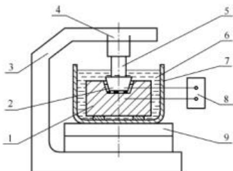
Schematic diagram of electrochemical polishing 电化学抛光示意图
