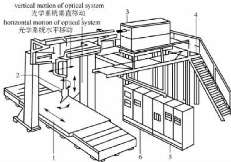
Laser beam machine 激光加工机
