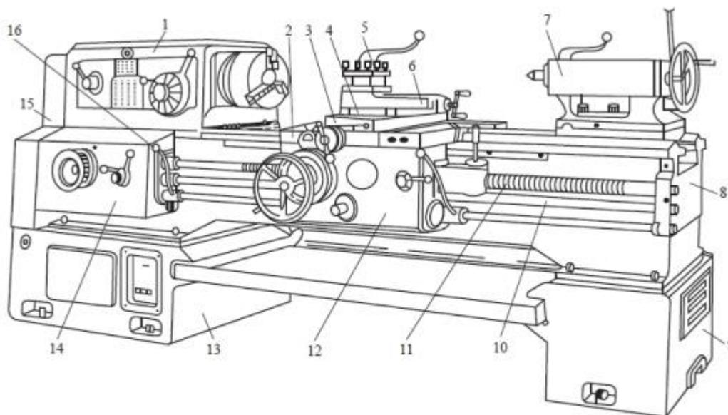
Layout of a general purpose horizontal lathe 卧式车床外形
