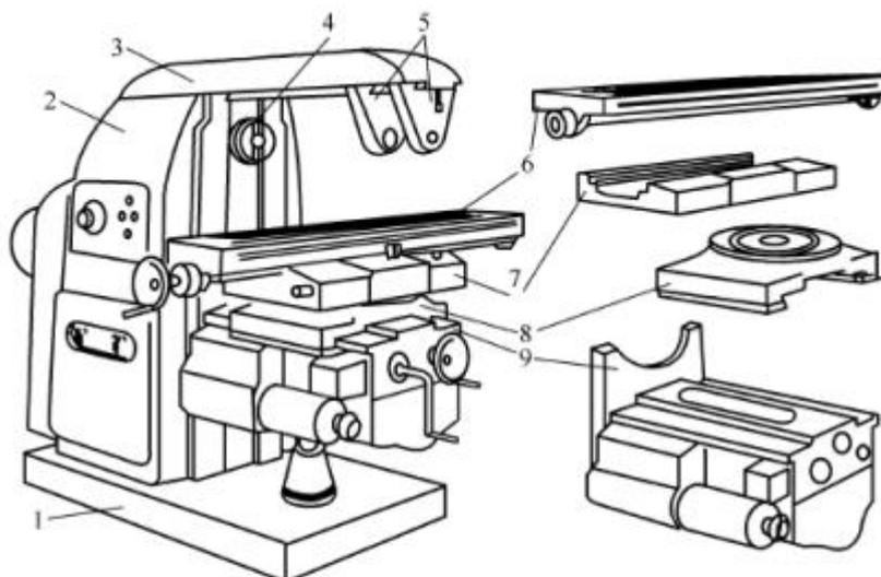
Horizontal knee and column type milling machine 卧式升降台铣床
