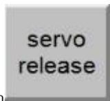
Click this button, the motor is switched between excitation and release to release the state, and the motor can be pushed by hand.
