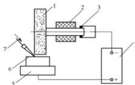
Schematic diagram of an electrochemical grinding operation 电解(电化学)磨削示意图
