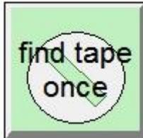
When the motor is energized and the tape and color sensor are normal, in manual mode, click to search for glue.
