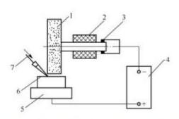
Schematic diagram of an electrochemical grinding operation 电解(电化学)磨削示意图
