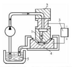
Principle of electrolysis(electrochemical machining) 电解(电化学)加工原理
