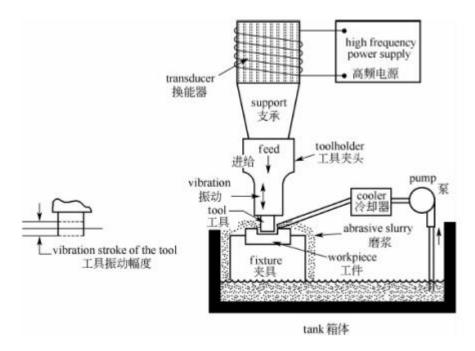
Schematic diagram of an ultrasonic machining operation 超声加工原理图
