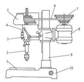
Drill press used on bench 台式钻床
