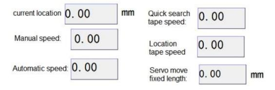
Set the servo auto, manual speed and quick find glue speed, glue speed and servo length.
